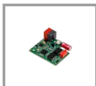
X.BE Electronic interface board between the KNX communication system and Beninca automations.
